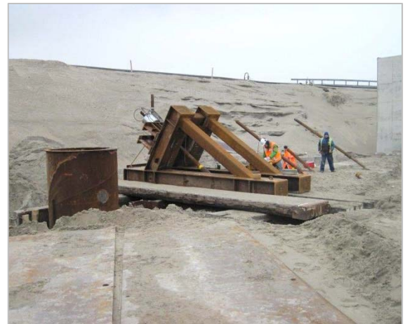
Testen groutankers Maasvlakte 2
